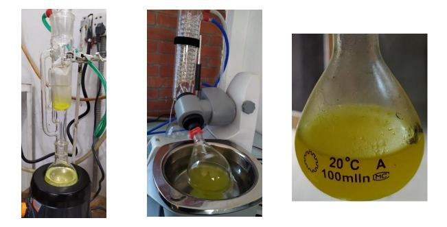
Figure 2.4: a) Extraction of fat by Soxhlet Apparatus;
