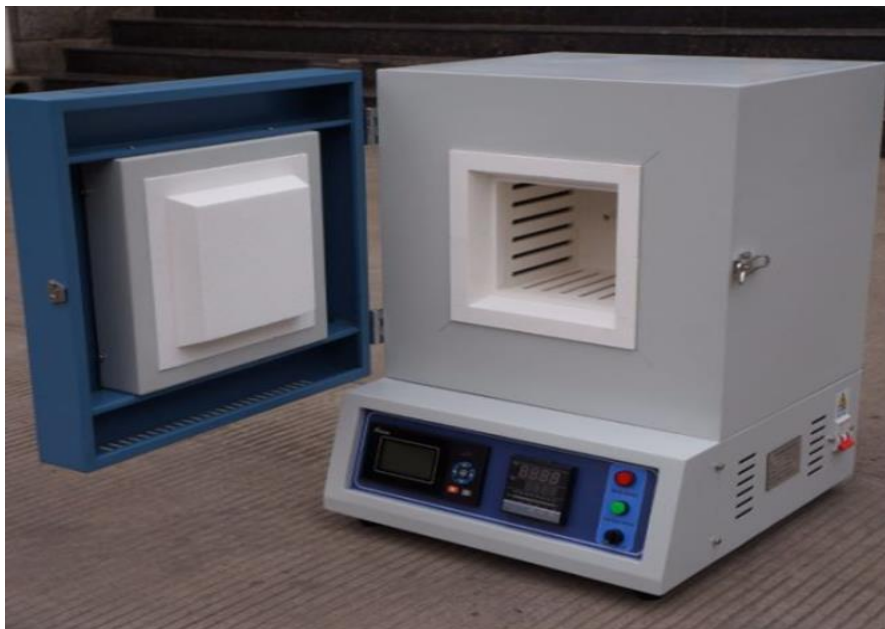
Fig-7: Muffle furnace
