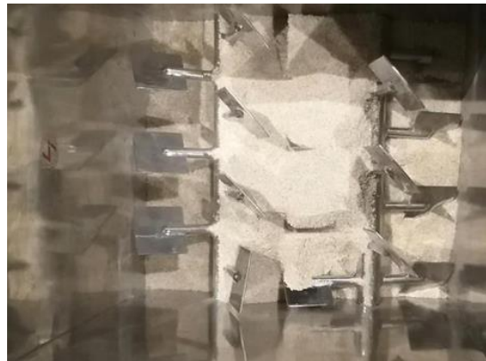
Figure 13: A) Forberg blender: A batch blender with paddle arrangement; B) Inside view of a Forberg blender
