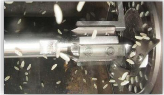
Figure 11: Cutting process with cutter
