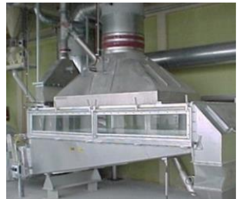
Figure 12: Fluid bed dryer
