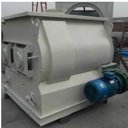
Figure 13: A) Forberg blender: A batch blender with paddle arrangement; B) Inside view of a Forberg blender
