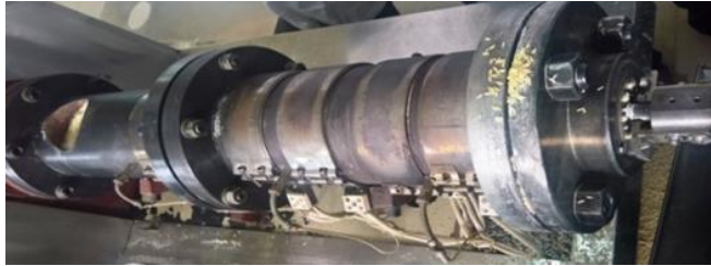
Figure 8: A Barrel with electrical heat Source
