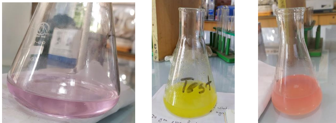
Figure 2.3: (Acid Value Determination) a) Blank Solution after Neutralization; b) Sample Solution before titration; c) Sample solution after titration
