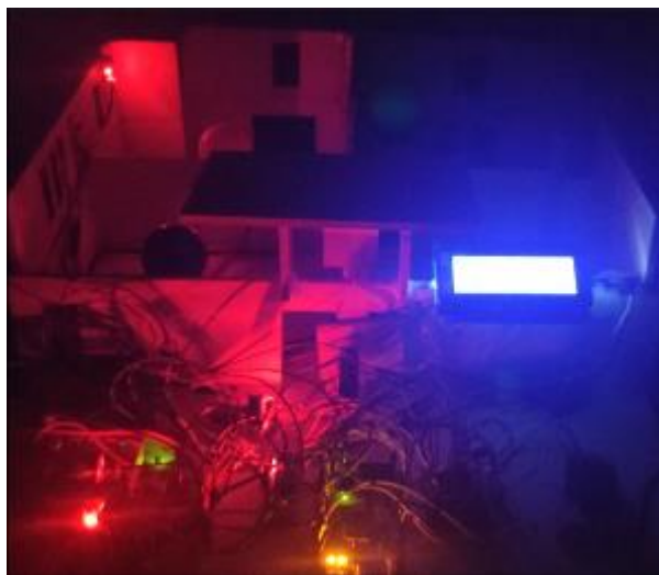
Fig 6.2.5: Controlling the loads with LDR sensor
