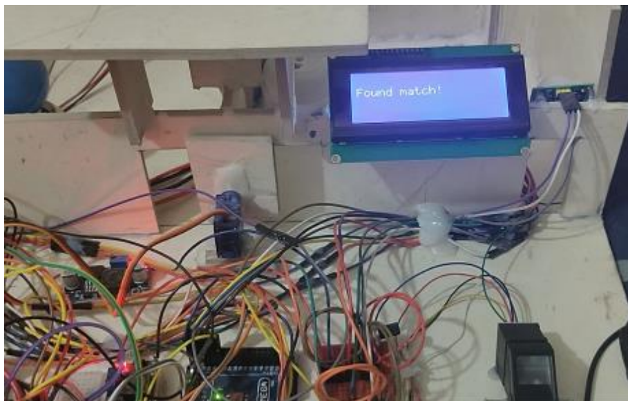
Fig 6.2.2: Opening the door when match found
