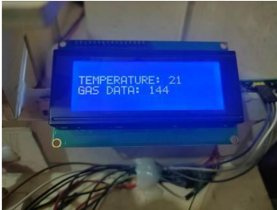
Fig 6.2.8: LCD display showing the temperature and gas data of the environment
