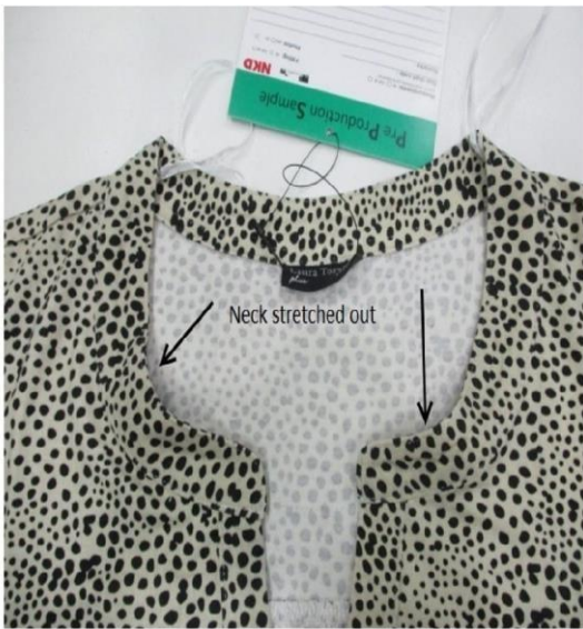
Fig. 3.87. Defect of PO 10060314
