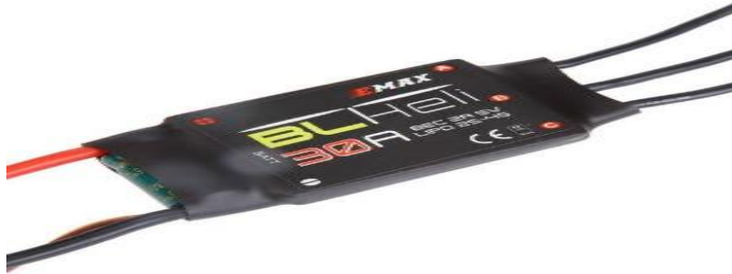
Figure 3:9 EMAX BL-Heli Series 30A ESC
