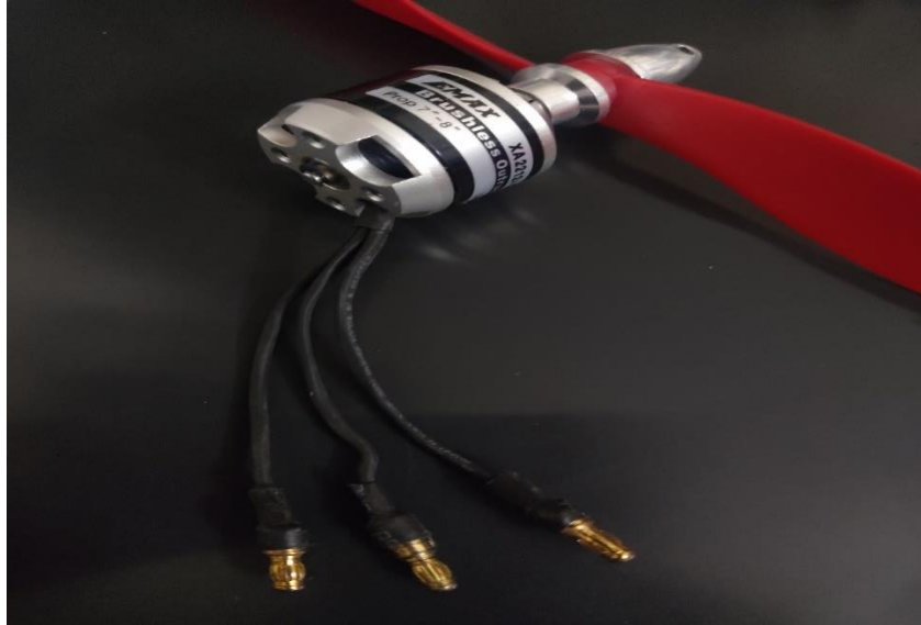
Figure 4:3 after bullet connection adding in BLDC
