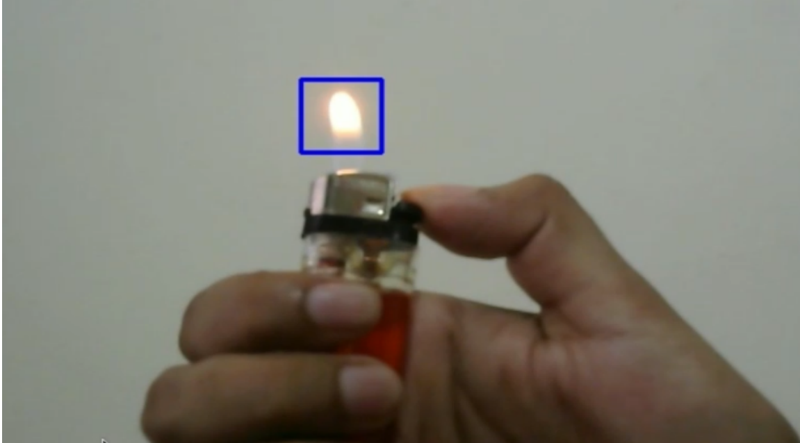
Figure 4.4: Fire Detection from Live Web Camera
