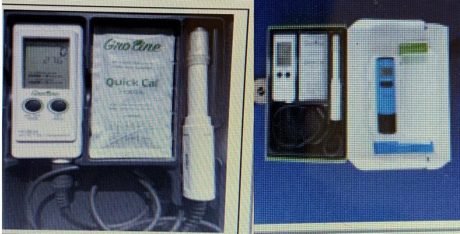
Tools we used to measure parameters including TDS and EC.
