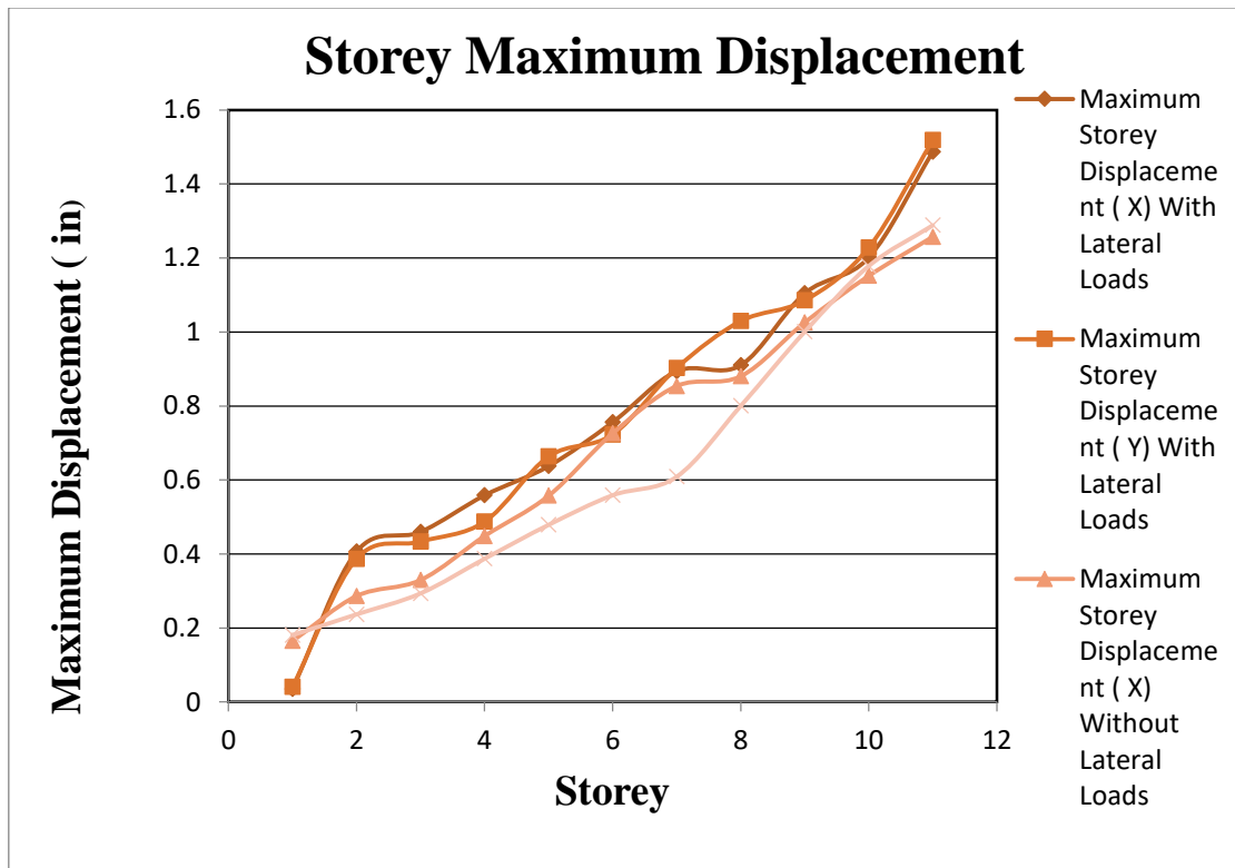
Fig. 5.1: Storey maximum displacement
