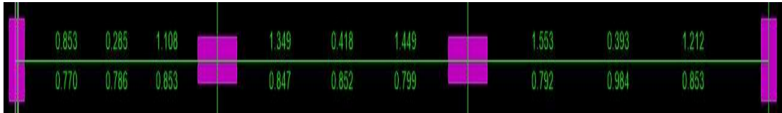
Figure 5.5: Reinforcement Area of 1 ST FLOOR (X-Axis)
