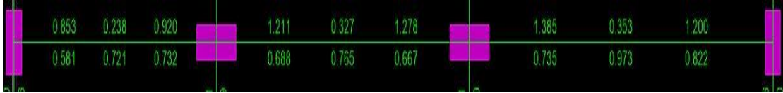
Figure 5.9: Reinforcement Area of 2 nd FLOOR (Y-Axis)
