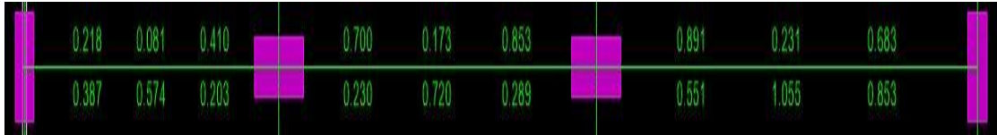
Figure 5.21: Reinforcement Area of Roof (X-Axis)
