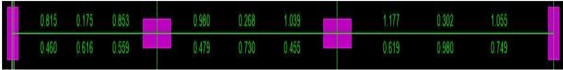
Figure 5.13: Reinforcement Area of 3 rd FLOOR (X-Axis)
