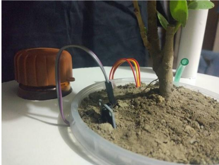
Figure 4.1.2: installation of soil moisturizer sensor
