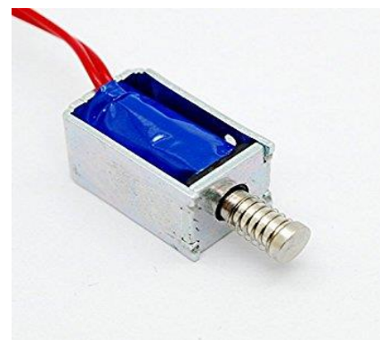
Figure 2.5: An Electromagnetic Solenoid
