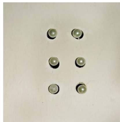
Figure 2.14: Top view of the refreshable display
