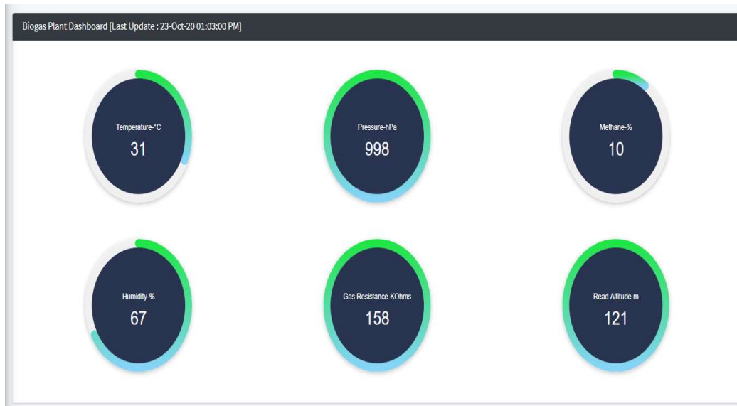
Figure 1.6.1: Application Dashboard contain latest Temperature, Pressure, Humidity, Gas Resistance, Read Altitude, Methane.
