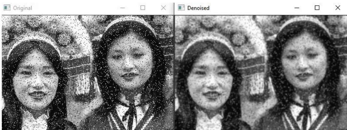
Figure 2.6.2.1: Before and after reducing salt n pepper noise by Gaussian filter
