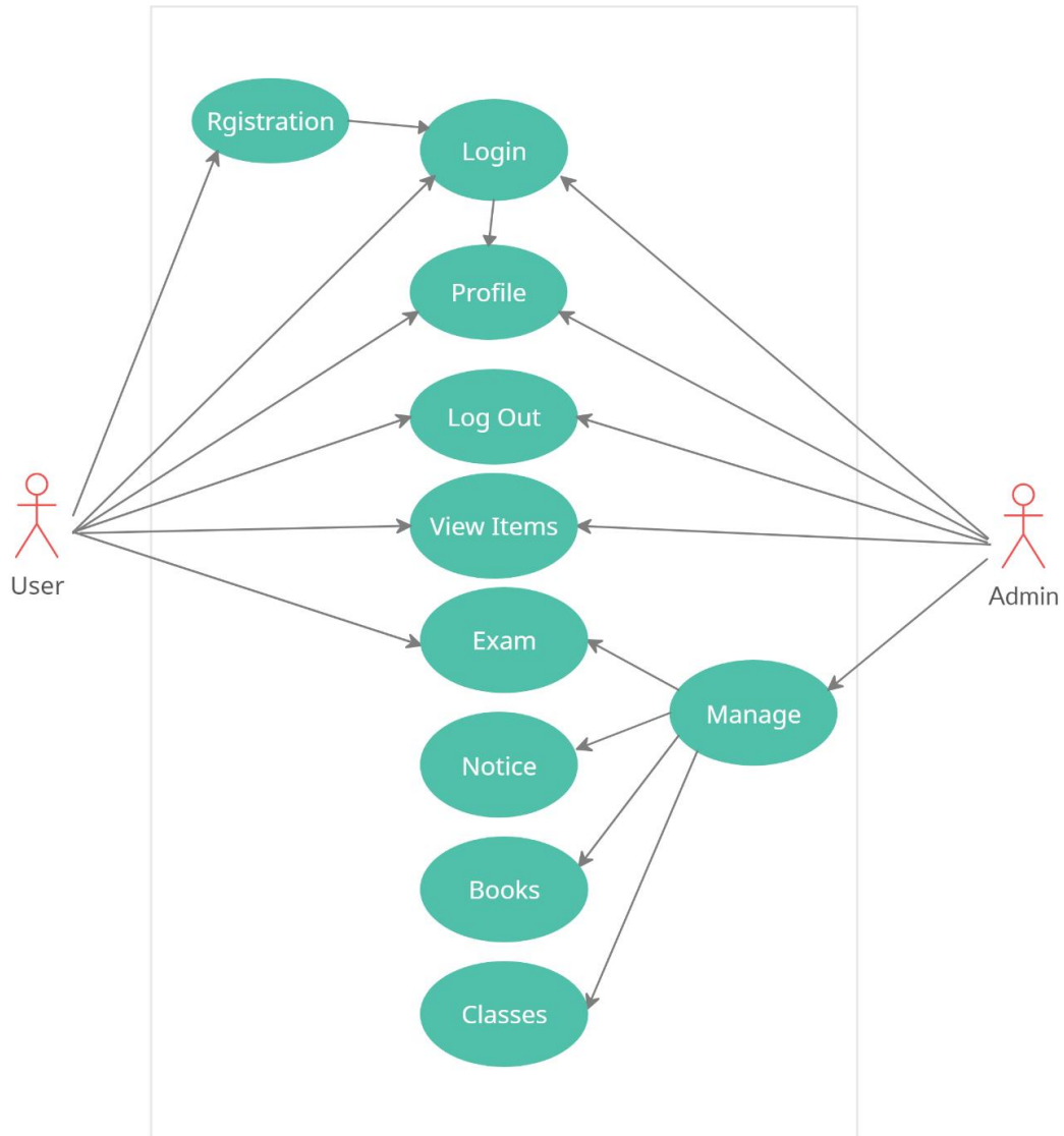
Figure 3.4: Use Case Diagram of Online Exam Management System
