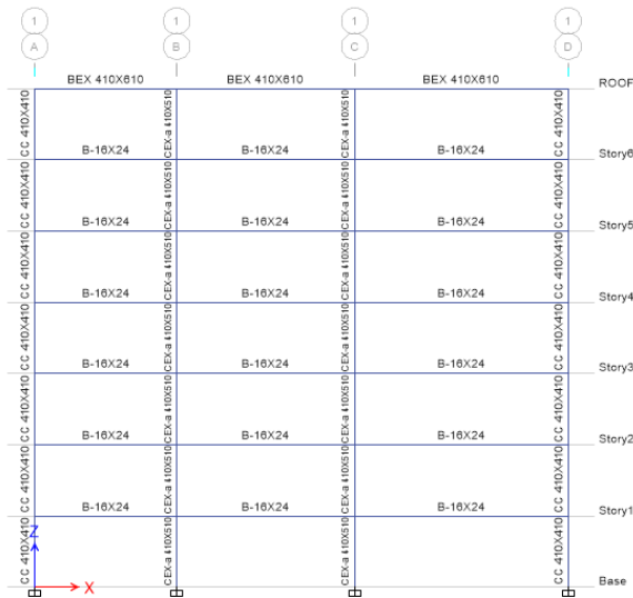
Fig 4.1: Grid 1A,1B,1C and 1D Column Position Layout
