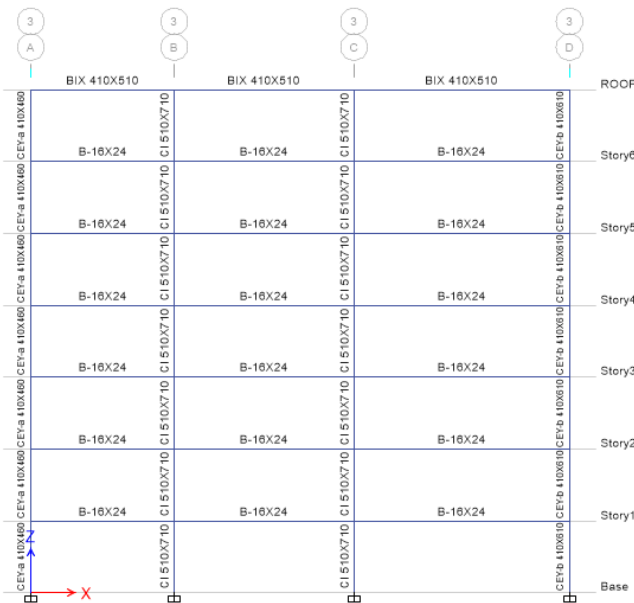
Fig 4.3: Grid 3A,3B,3C and 3D Column Position Layout
