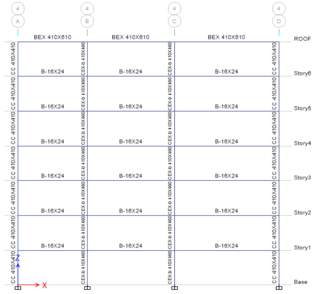
Fig 4.4: Grid 4A,4B,4C and 4D Column Position Layout
