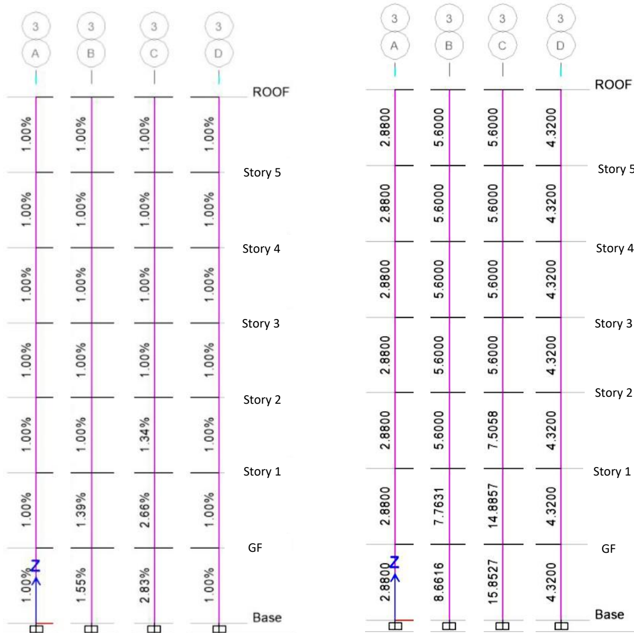
Fig 8.10: Grid 3 Rebar Percentage & Area
