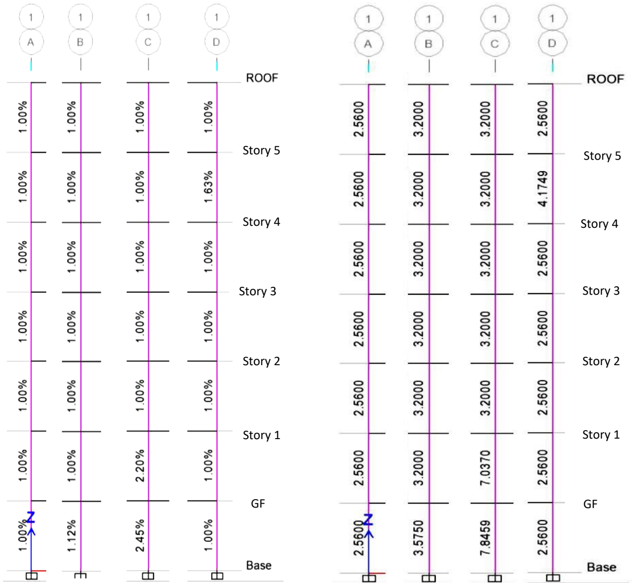
Fig 8.8: Grid 1 Rebar Percentage & Area
