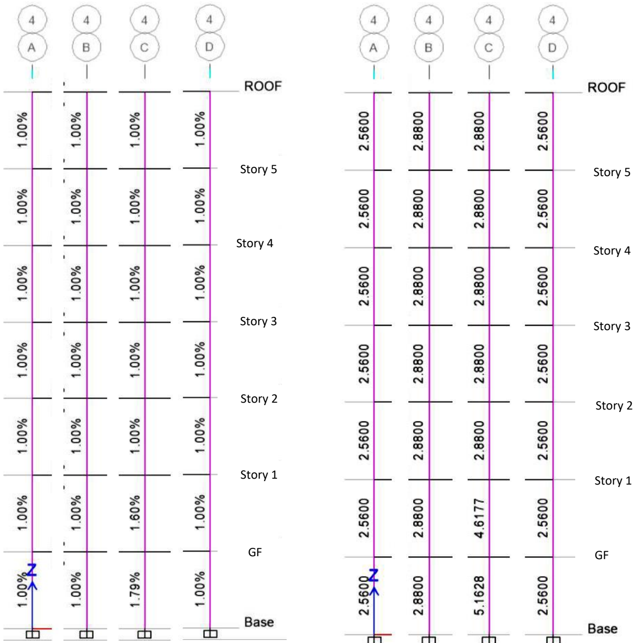
Fig 8.11: Grid 4 Rebar Percentage & Area
