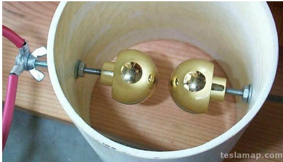
Fig. 4.7: Static spark gap [30]
