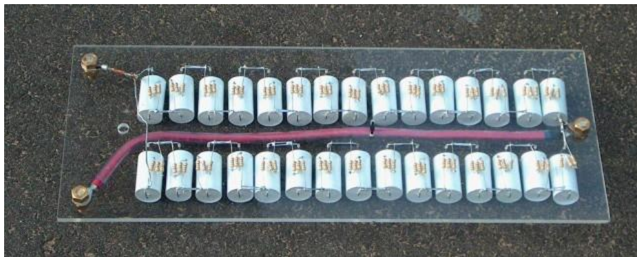
Fig. 4.6: Typical MMC array [30]
