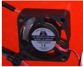
Figure 4.7: Air cooling unit
