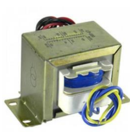
Figure No 4.2: Center tapped Transformer
