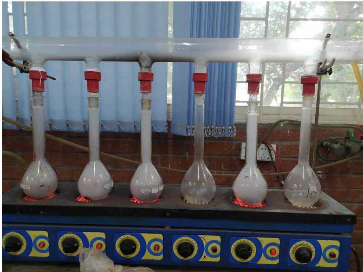
Figure 13: Digestion flask heated in a kjeldahl digestion chamber.
