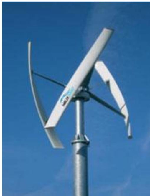
Fig 3.4: Vertical axis wind turbine
