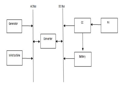
Fig 4.1: Block diagram of system design.
