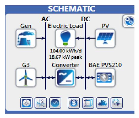
Fig 4.2: Hybrid mini-grid system design by homer software.
