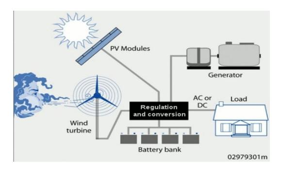
Fig 1.11: Hybrid mini-grid system model.
