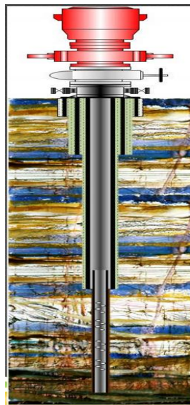
Figure 4.12: Slim Well Drilling [10]
