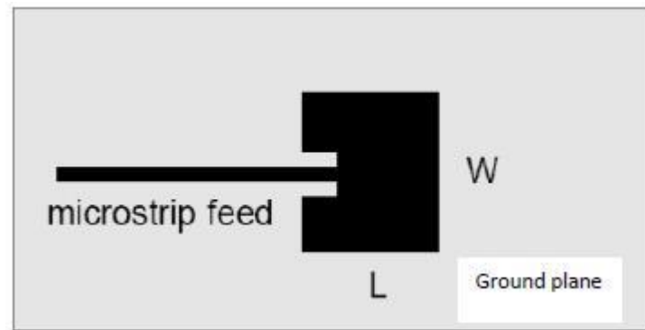
Figure 2.9 Microstrip feeding of patch antenna
