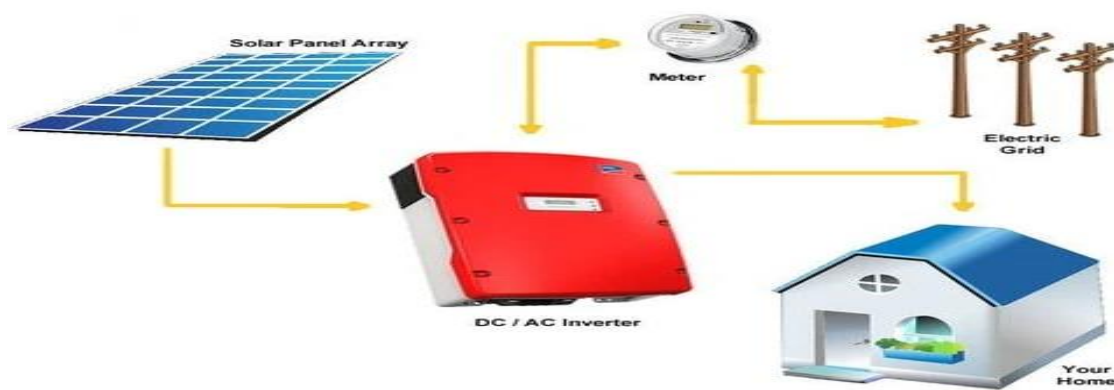
Fig.2.7: On grid solar rooftop system
