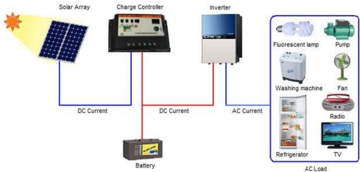
Figure 6.2: Circuit of Solar Home system
