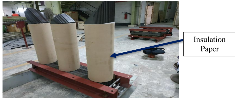
Figure 4.8: Insulation paper and bottom Separator
