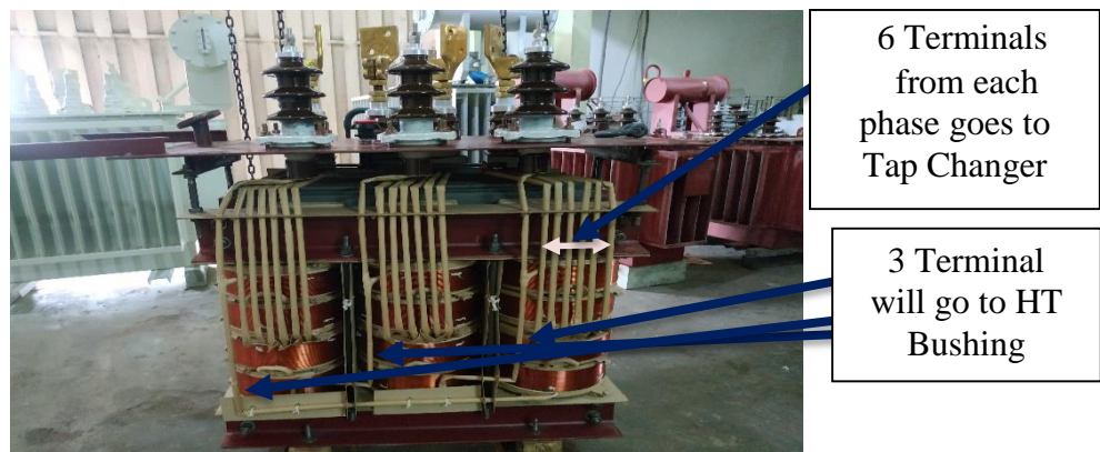
Figure 4.12: Delta Connection
