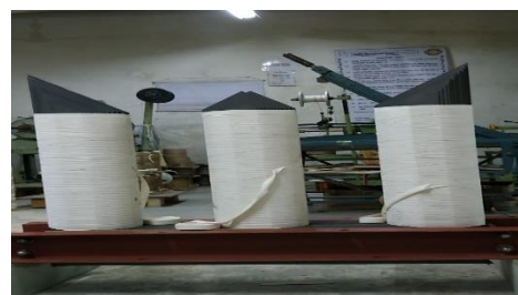
Figure 4.7: Cotton tape sprayed above core
