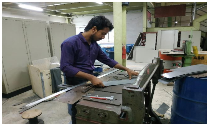
Figure 4.4: Cutting Core 450 for MITRED shape
