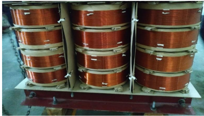
Figure 4.10: Core Coil (HT & LT) Assembling
