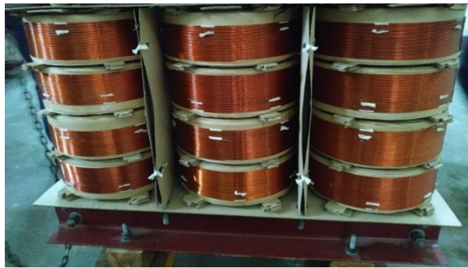
Figure 4.10: Core Coil (HT & LT) Assembling
