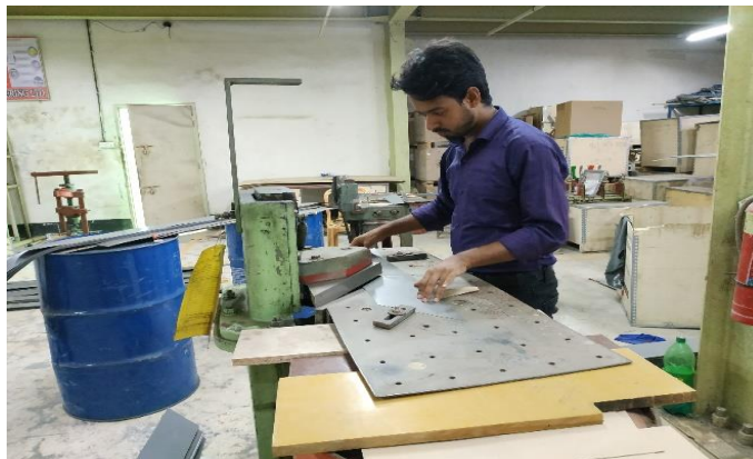
Figure 4.3: Cutting “V” notch in Core B
