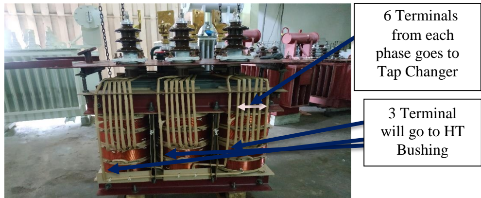
Figure 4.12: Delta Connection
