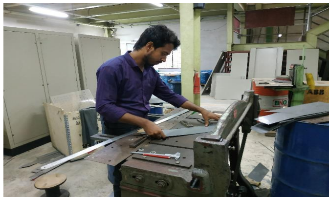
Figure 4.4: Cutting Core 45° for MITRED shape
