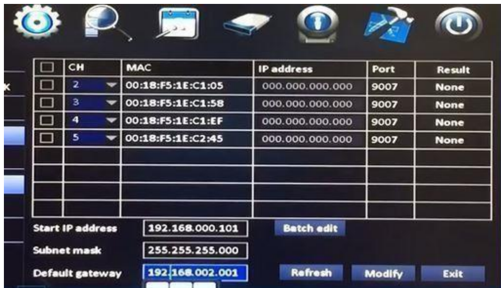
Figure:5.6 IP address Subnet Mask and gateway
