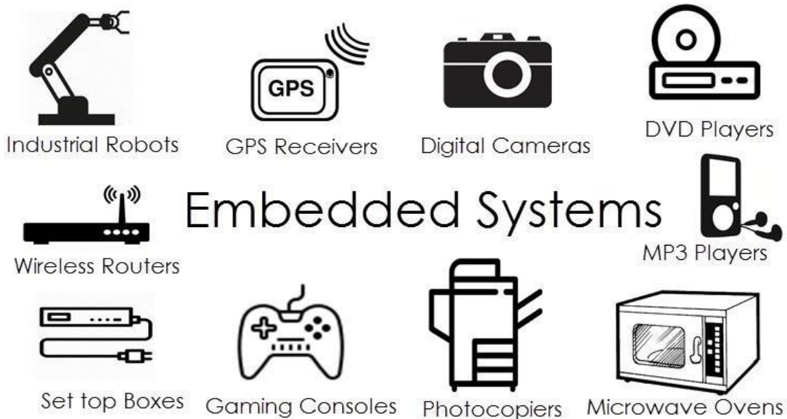
Figure3.1.3:Examples of Embedded Systems
