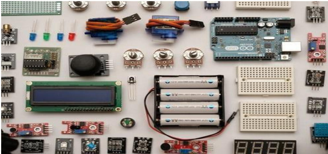
Figure3.1.2:Arduino Starter Kit
