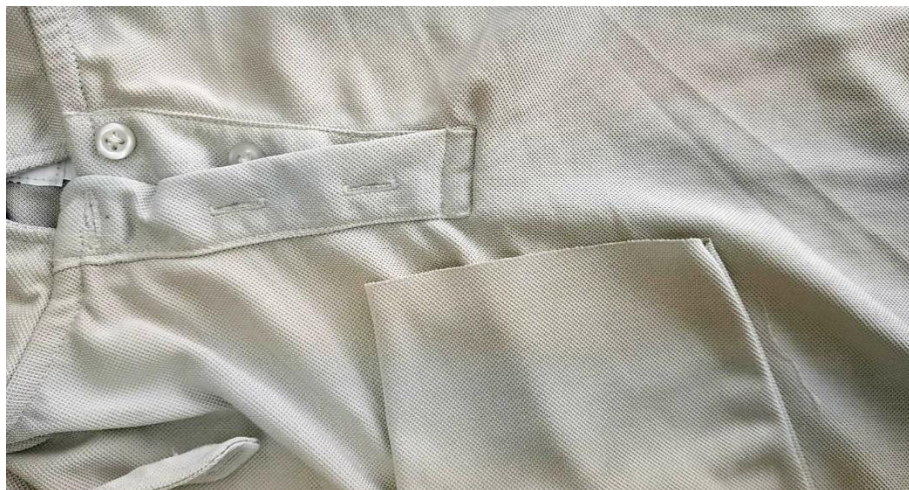
Fig: Cuff Missing
