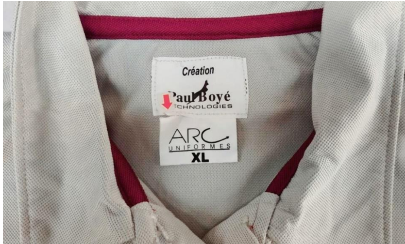
Fig: Improper Size Label Joining
