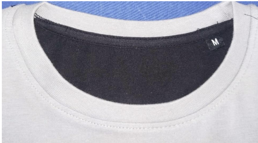
Fig: Main Label Missing
