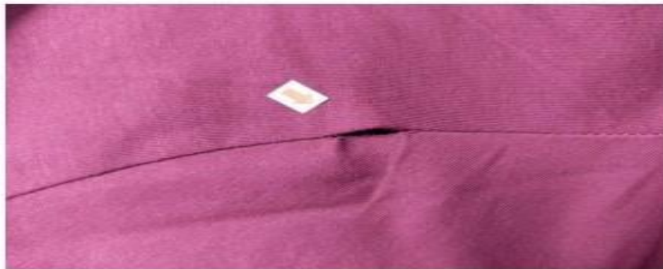
Fig: 2.6.11 – arm hole joint problem
