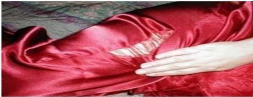
Fig: 2.6.6 - Seam slippage
