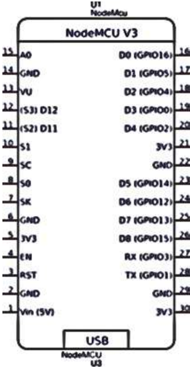
Fig. 3.4.4: Circuit diagram of NodeMCU (ESP8266)
