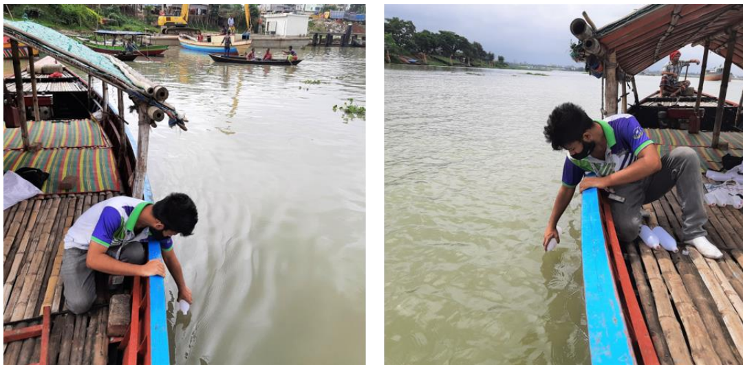
Photograph: On field water sample collection from Turag River using a motor boat.
