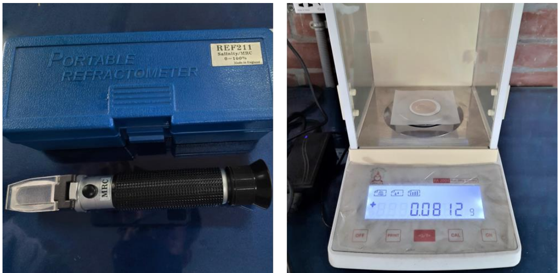
Photograph: Salinity meter & analytical weight balance at ESDM Lab.
