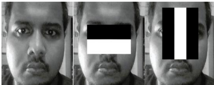
Fig 3.4: Feature detection by applying Haar features
