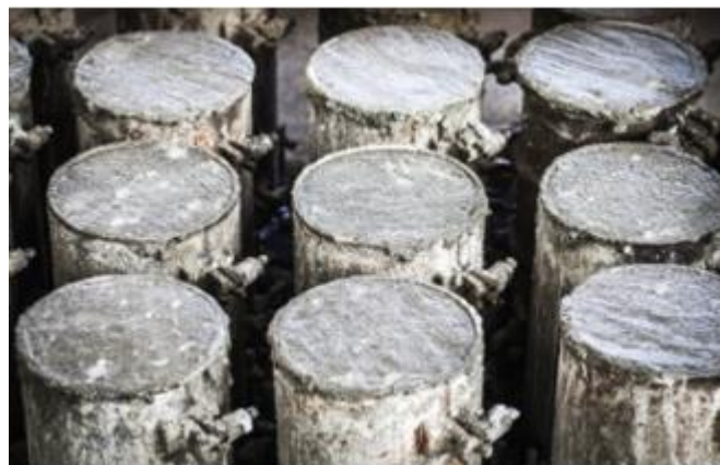
Figure 3.9: Casted Concrete in molds
