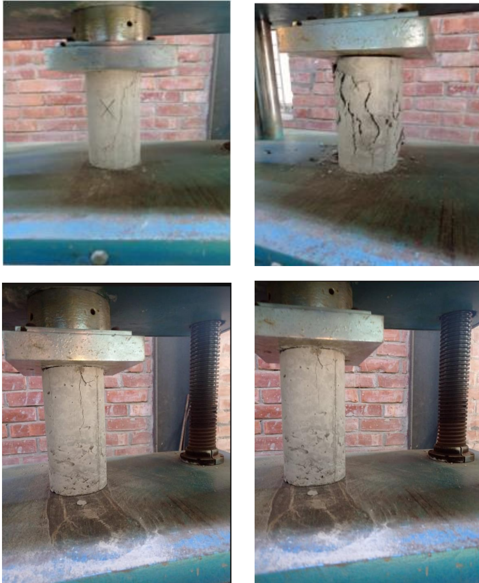
Figure 3.18: compressive strength test of cylinder mold
