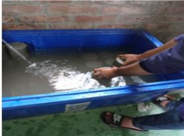
Figure 3.11: Replacing the water at Curing
