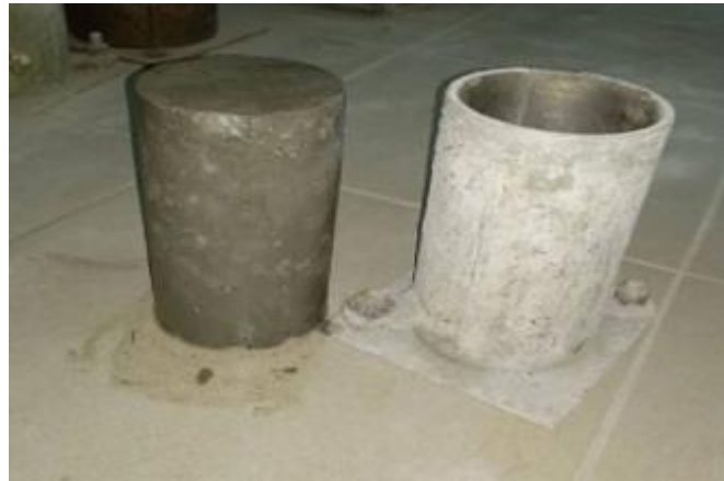
Figure-3.12: Opening Cylinder Specimen from Molds
