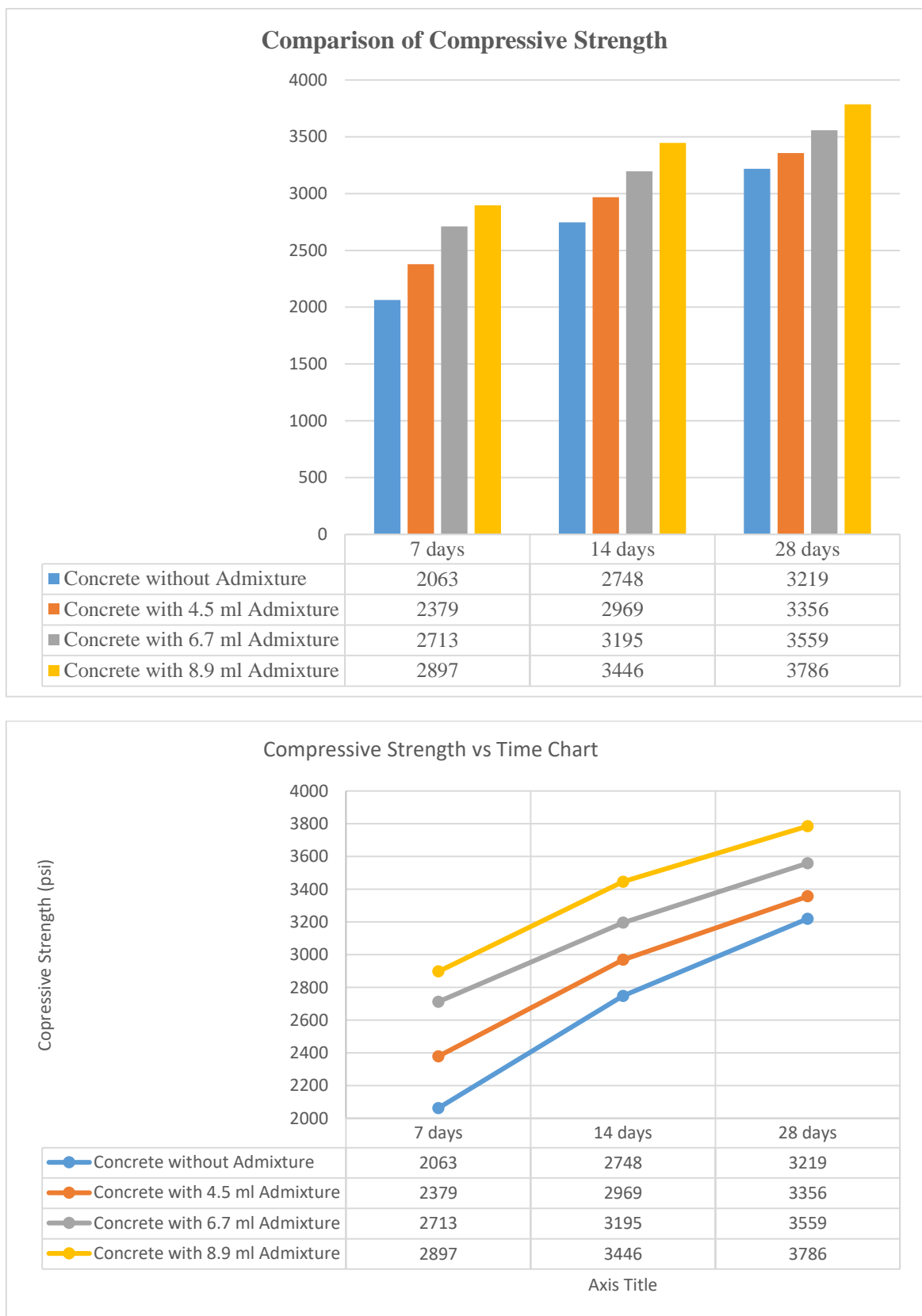
Figure-4.7: Comparison Compressive Strength VS Time Curve
