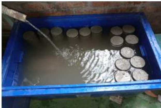
Figure 3.10: Curing of cylinder molds
