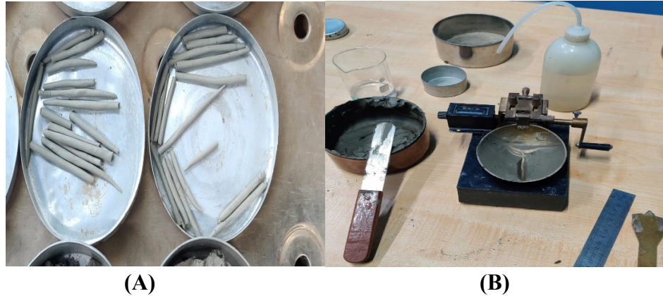
Figure 46: (A) Plastic limit & (B) Atterberg limit test
