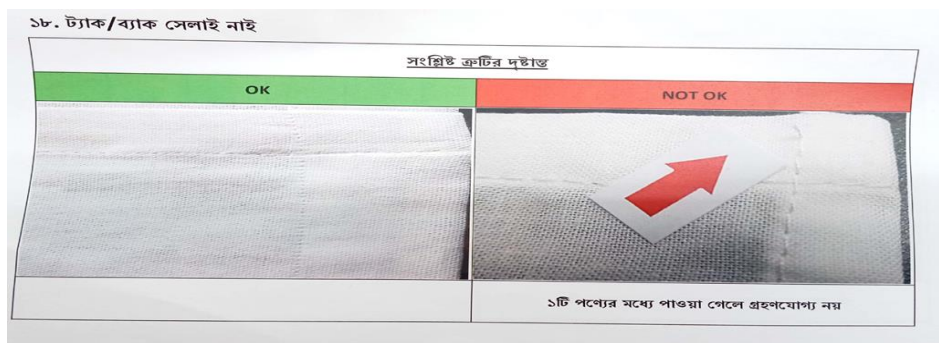
Fig 05: Back stitch Missing
