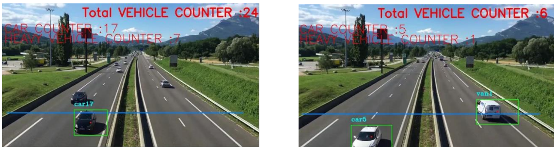
Fig-9: vehicle detection, counting & classification
