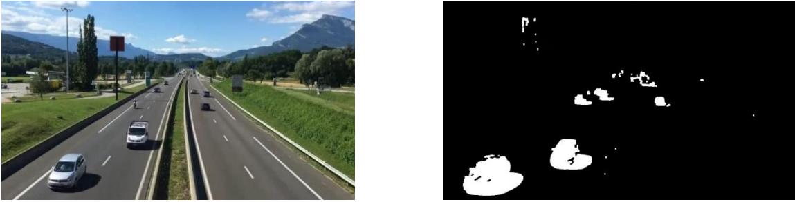
Fig 5: Using subtractor Algorithm
