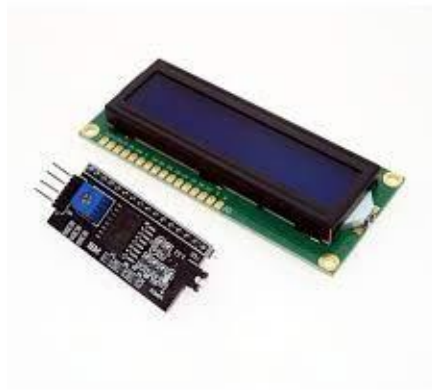
Figure 3.7 : LCD display with i2c
