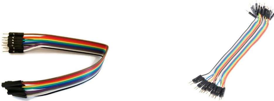
Figure 4.10(a) Female to Male Jumper Wire. Figure 4.10(b) Male to Male jumper wire.
