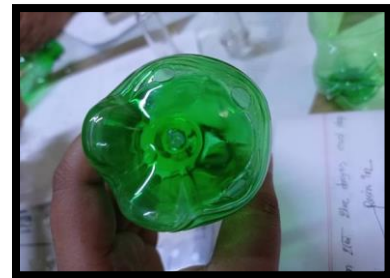
Figure-8: Faulty Preform
