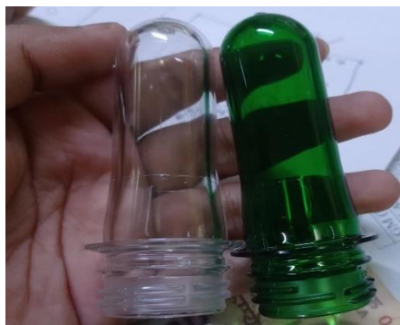
Figure-5: Picture of 250 ml bottle preform.
