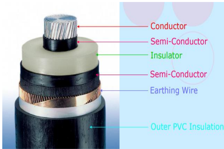
Figure 3.13.1 Cross - Sectional view of Power Cable
