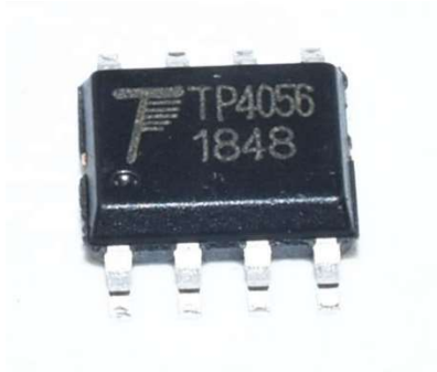
Figure 5.7: TP4056 Constant-Current/Constant-Voltage Linear Charger IC
