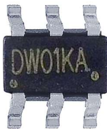
Figure 5.8: DW01A Battery Protection IC
