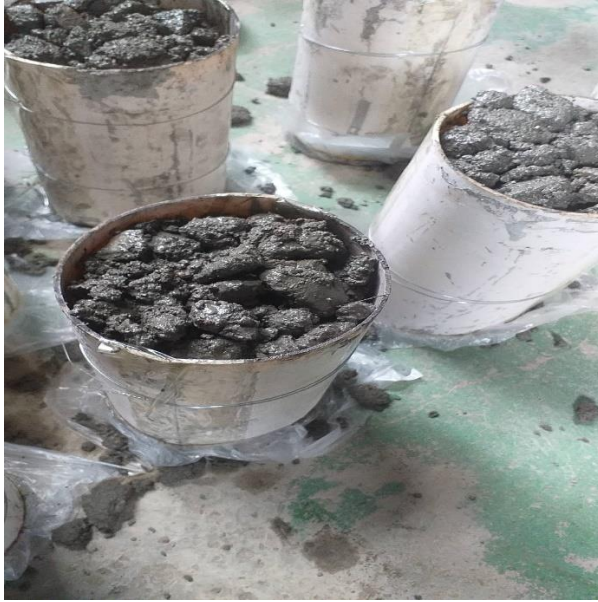
Fig 3.6: Casting the mold with concrete.
