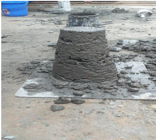
Fig 3.3: Slum Cone Test
