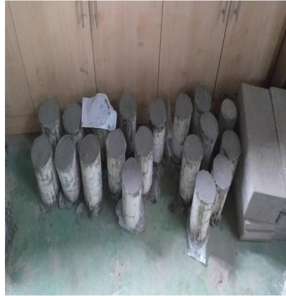
Fig 3.6: Casting the mold with concrete.
