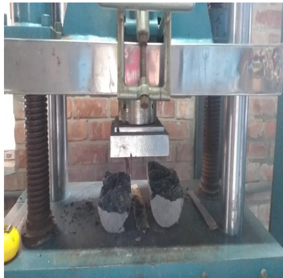
Fig. 3.8: Split Tensile Strength Test
