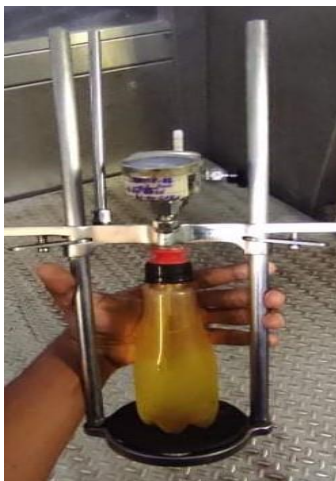
Fig 24: Gas Volume Test
