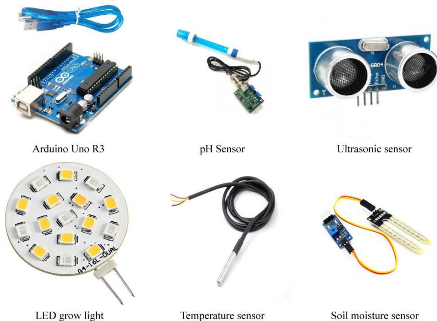
Fig 5.1: Sensors Using in Smart Indoor Gardening
