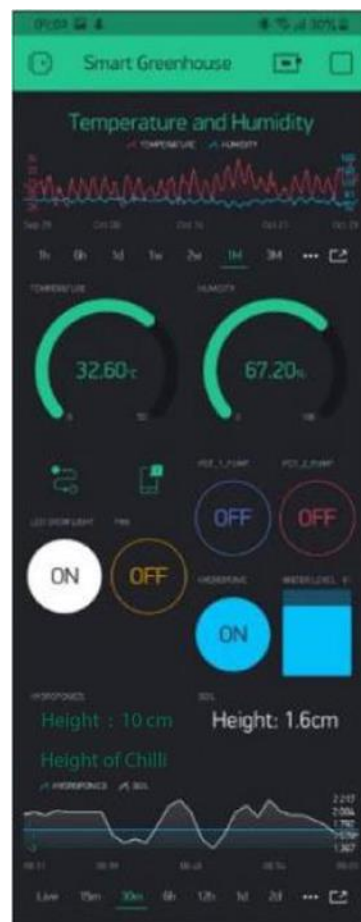
Fig 7.1: shows how the Blynk app works on a mobile phone
