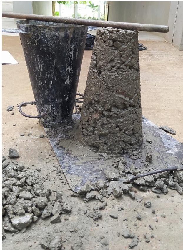
Figure 4.1: Slump test results = 0
