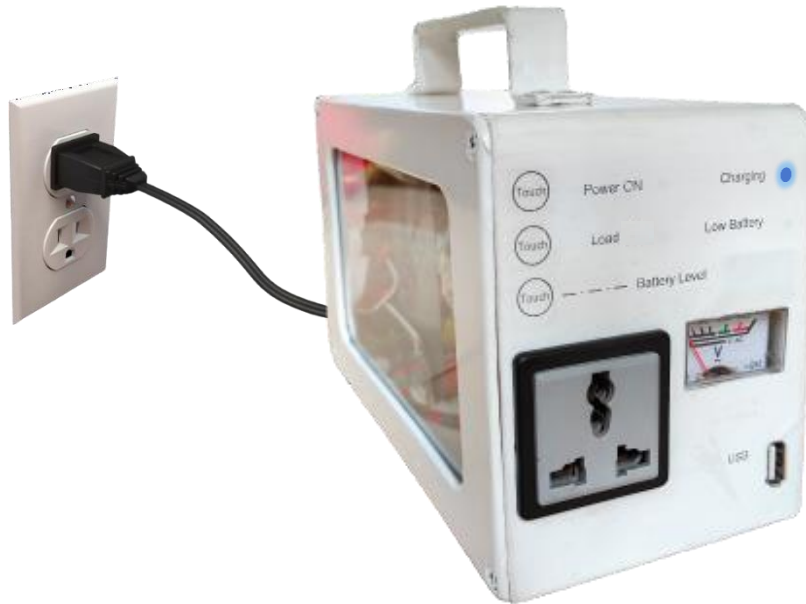
Fig.5.2.8 Portable IPS battery charging view
