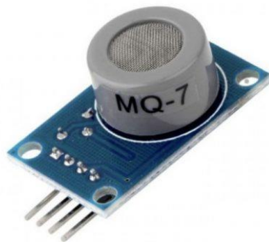
Fig-9: MQ-07 sensor.
